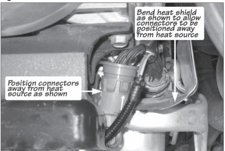
Figure 4 Grounding Location & Black Intercepting Connectors Shown
