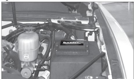
Figure 10 Placement of the Banks Brake Module
