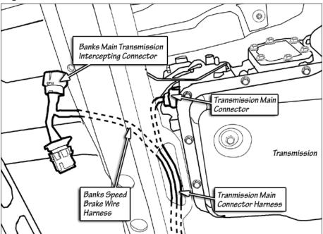
Figure 2 Main Transmission Connector Location
