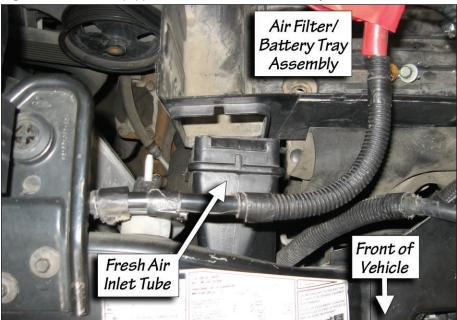
**10.** Remove the factory battery tray and air filter box assembly from the vehicle.
