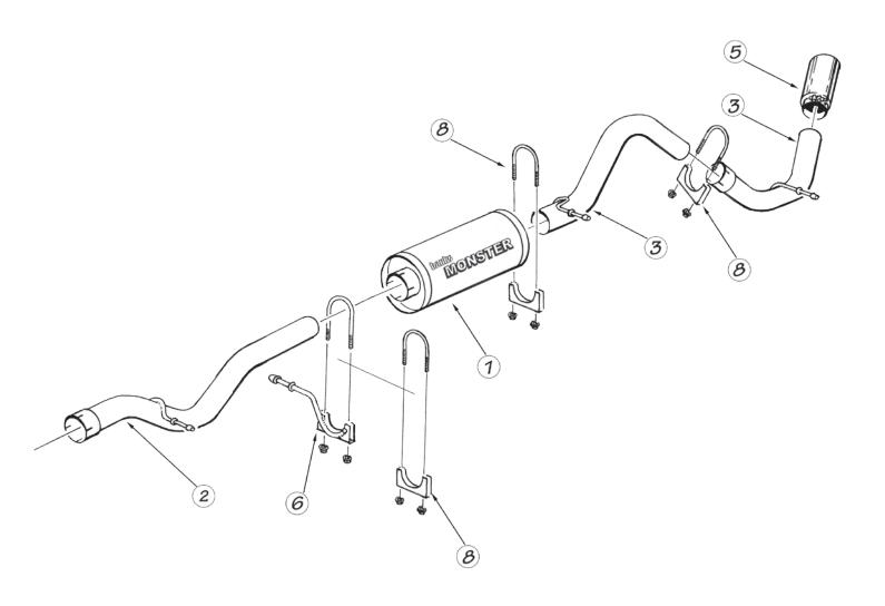
Figure 1b General Assembly Banks Split-Dual Monster Exhaust, Split-Dual
