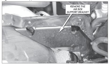
Figure 17 Before and after removing material from the air box support bracket.
