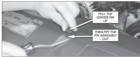
Figure 10a Headlamp assembly removal, Chevy
