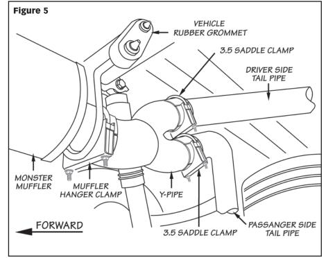
**13.** Insert the intermediate pipe inlet onto the flanged intermediate pipe outlet. Install the intermediate pipe hanger pin(s) into the vehicle rubber grommets.
