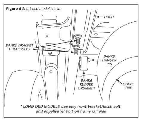
For Long bed models, use one (1) bolt on the flat of frame rail and one (1) bolt on the side of the frame rail.
