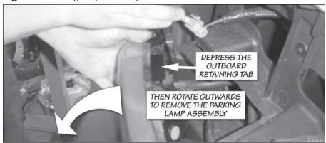
Figure 12 Removal of headlamp/parking lamp assembly support structures
