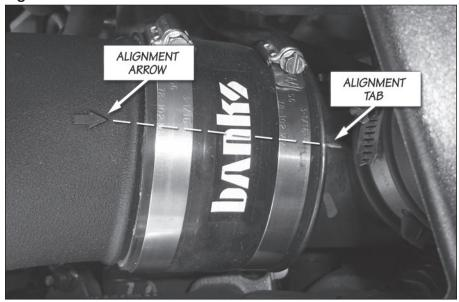
**10.** Locate the Banks Ram-Air filter and the Banks filter hose clamp. Loosely fit the Banks Ram-Air filter clamp to the Banks Ram-Air filter.
