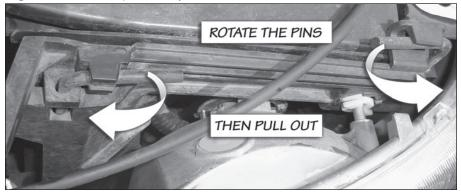
Figure 11 Parking lamp assembly removal
