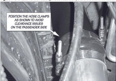
Figure 7 Orientation of the Passenger Side Hose Clamps to avoid clearance issues.
