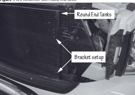
Figure 1 A/C condenser with round end tanks
