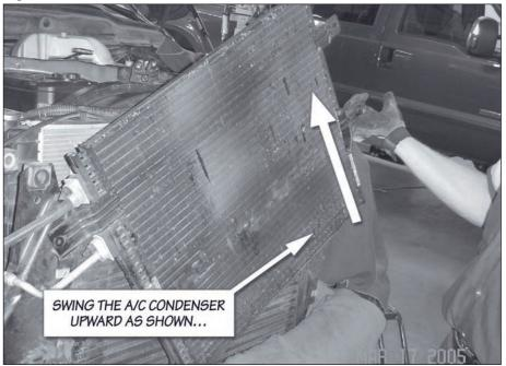
Figure 6 A/C Condenser Removal Procedure
