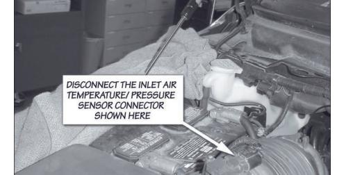
Figure 2 Location of the Inlet Air Temp/Pressure Sensor
