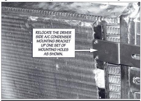
Figure 5 A/C Condenser Removal Procedure
