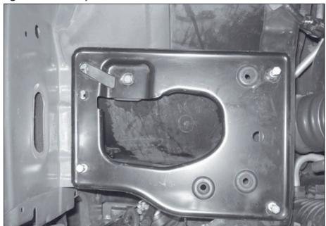
Figure 12 Air box support bracket
