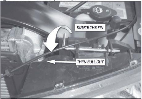
Figure 4 2006-07 LBZ: Parking Lamp Assembly Removal
