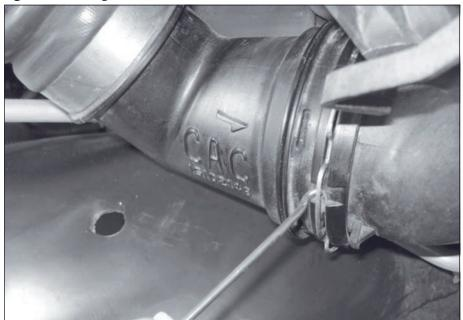
Figure 18 Passenger side boost tube
