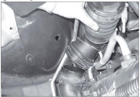
**27.** Remove the charge air cooler from the vehicle. Check that the lower mounting peg grommets are removed from the stock intercooler and place to the side. The lower rubber grommet will be transferred to the Banks intercooler in the next step.
