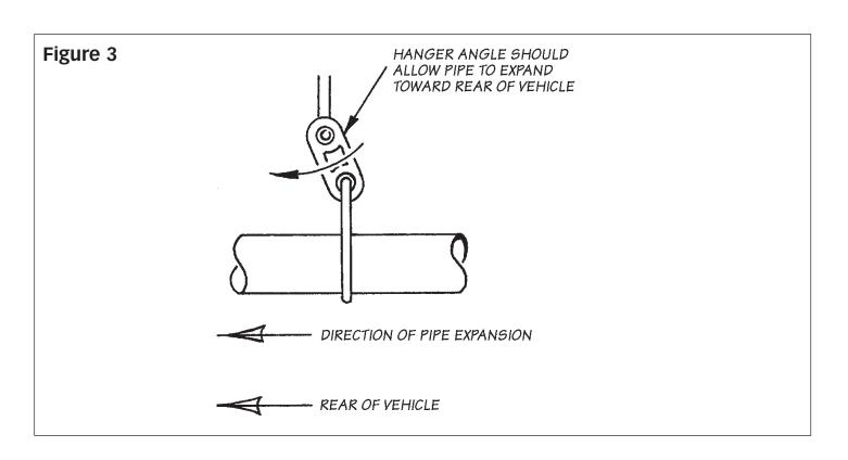
intermediate pipe. Temporarily support the muffler and install the hanger clamp at the front of the muffler. Snug the nuts, but do not fully tighten them.
