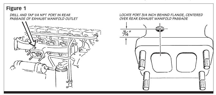
cause turbine blade damage. The Cummins ISB engine uses a divided exhaust manifold and turbocharger. The thermocouple may be installed to sample exhaust temperature in either exhaust passage. We recommend the rear passage (toward the firewall).
