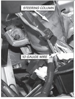
**41.** Locate the long gray wire on the Banks TCC wire harness. Route this wire with the factory wire loom across the base of the cowl and
