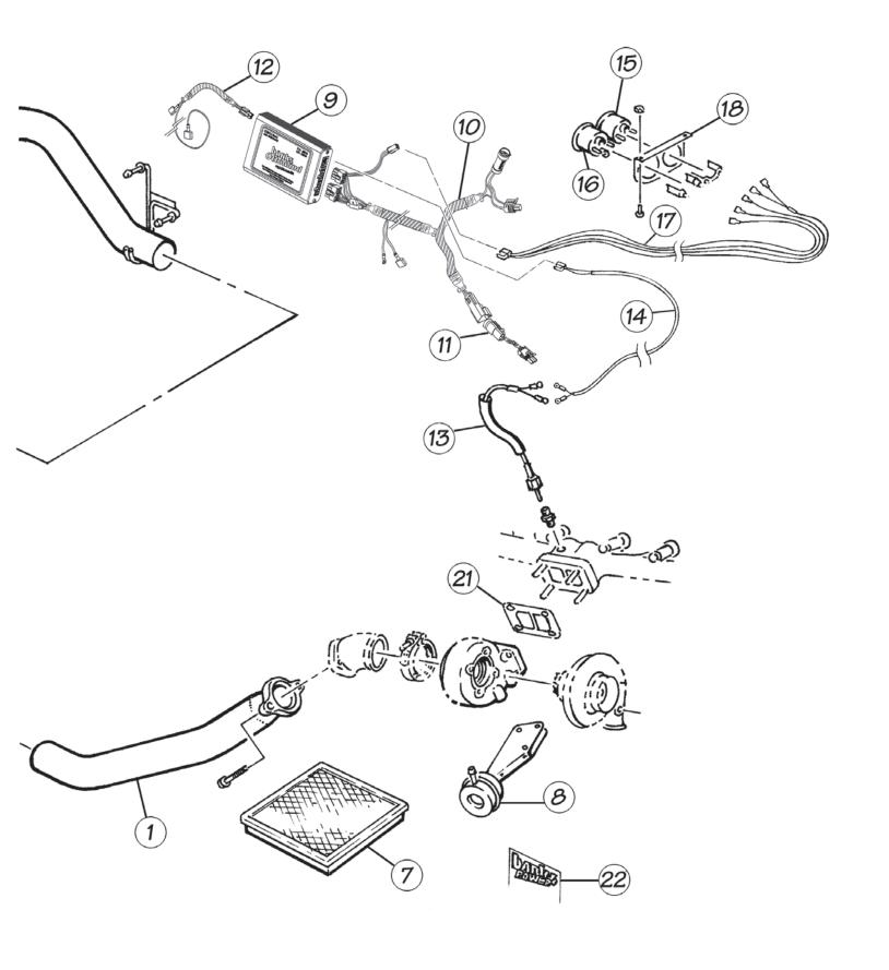
used, loosely bolt the bracket into place on the turbine housing with the actuator bolted to the bracket using the original locknuts.
