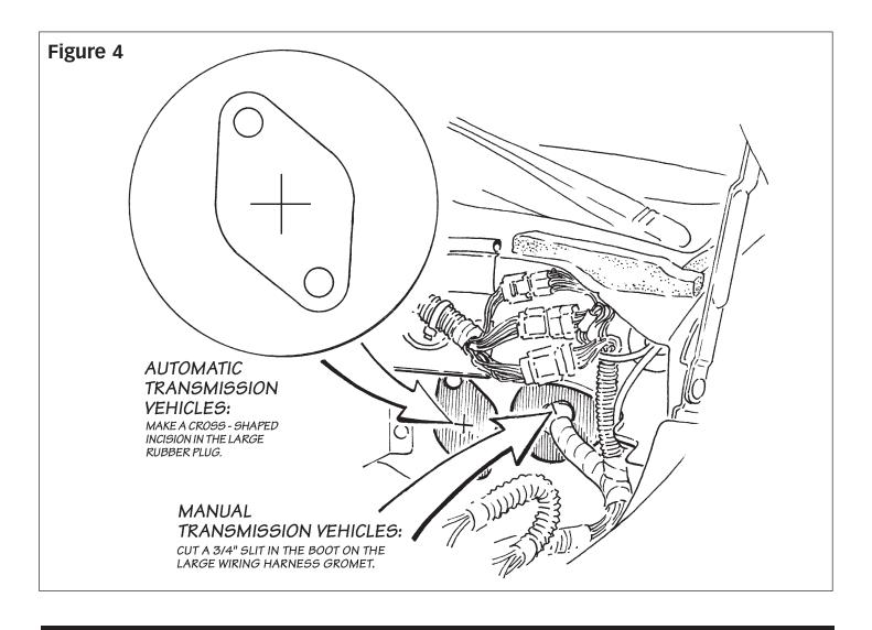
33. Insert the end of the provided OttoMind wire loom with the 8- and 10-pin connectors through the grommet from the engine compartment. Pull the Ottomind wire loom from inside the cab until approximately 18" of the wire loom is inside the cab.
