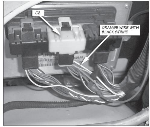
the triangular connector on the OttoMind wire harness, then follow 2001-2002 CAN BUS installation procedure.
