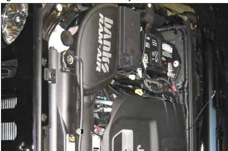
Figure 8- Installed Banks Ram-Air Intake System
