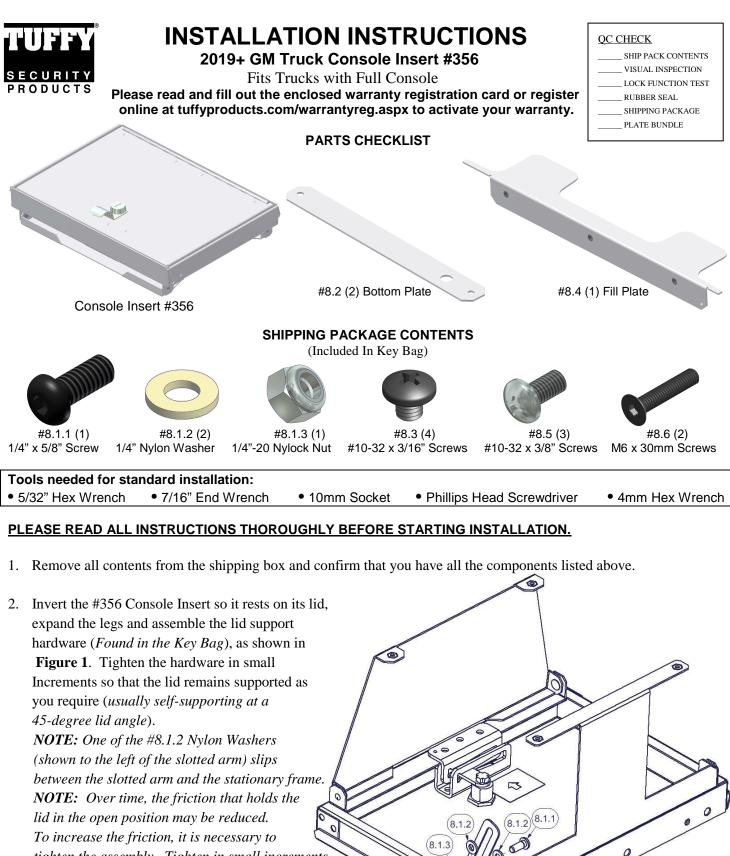
To increase the friction, it is necessary to tighten the assembly. Tighten in small increments as required, removal of the Console Insert should not be necessary.
